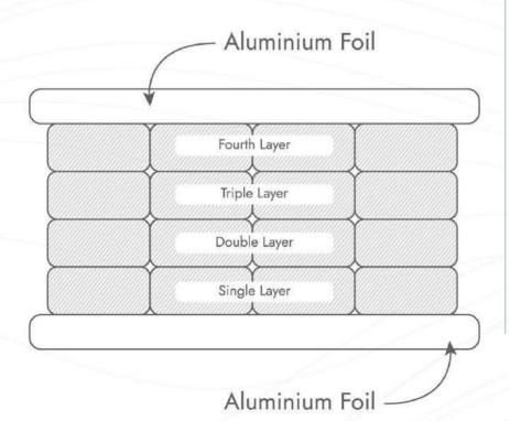
We manufacture **Air Bubble Insulation** with 97% reflection ratio, which are most preferred kind of insulations available in the market today. The thickness starts from 4mm, 6mm, 8mm, 10mm, 12mm, 16mm & 20 mm with single bubble, double, triple bubble & four layer of bubble. Material is laminated with single or both side aluminium foil, single or both side Metpet.
